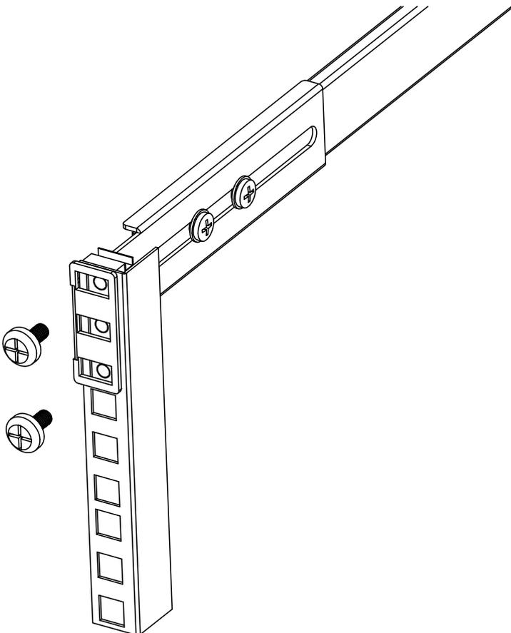
6. Pull the middle rails out of the slide rail assemblies.
