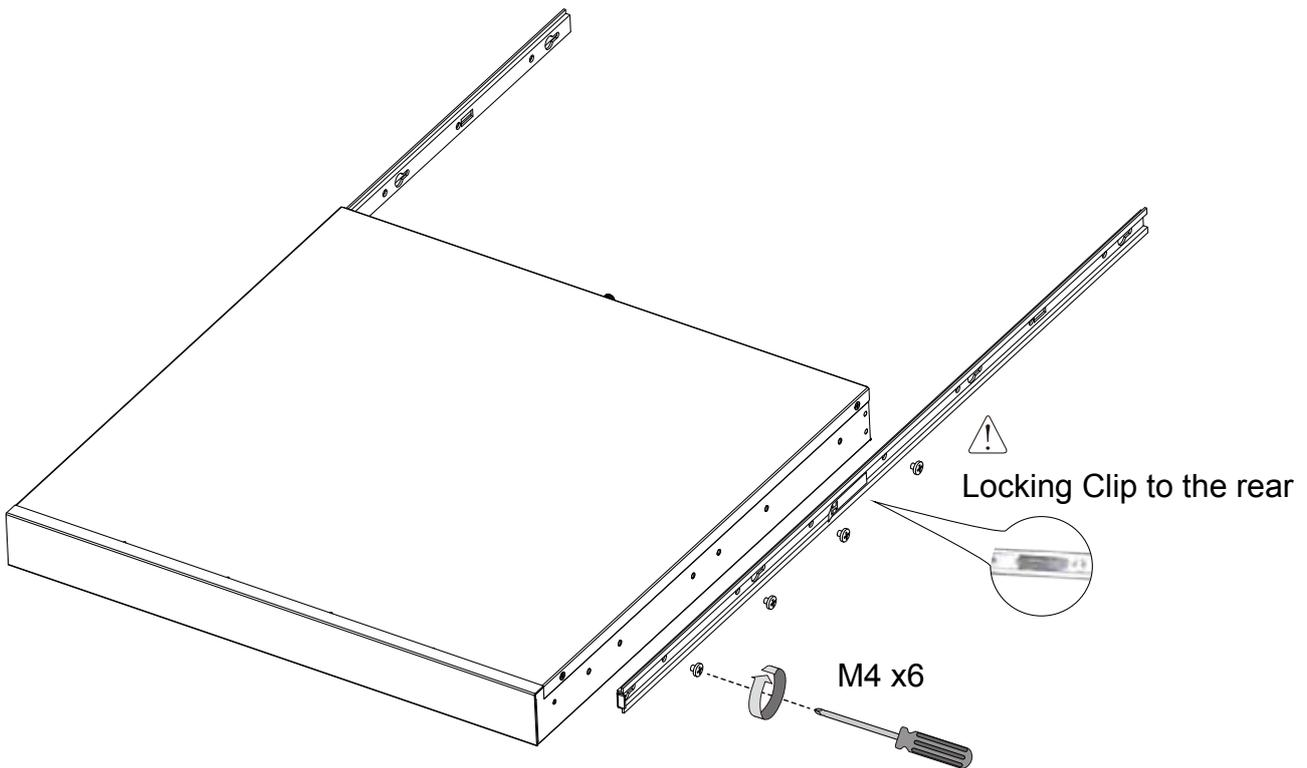
4. Secure the L-shape brackets to the front- and rear-ends of outer rails using the **black** round head screws and washers. Do not completely tighten the screws yet. Adjust the length of slide rails by extending and matching the rails between rack posts.
