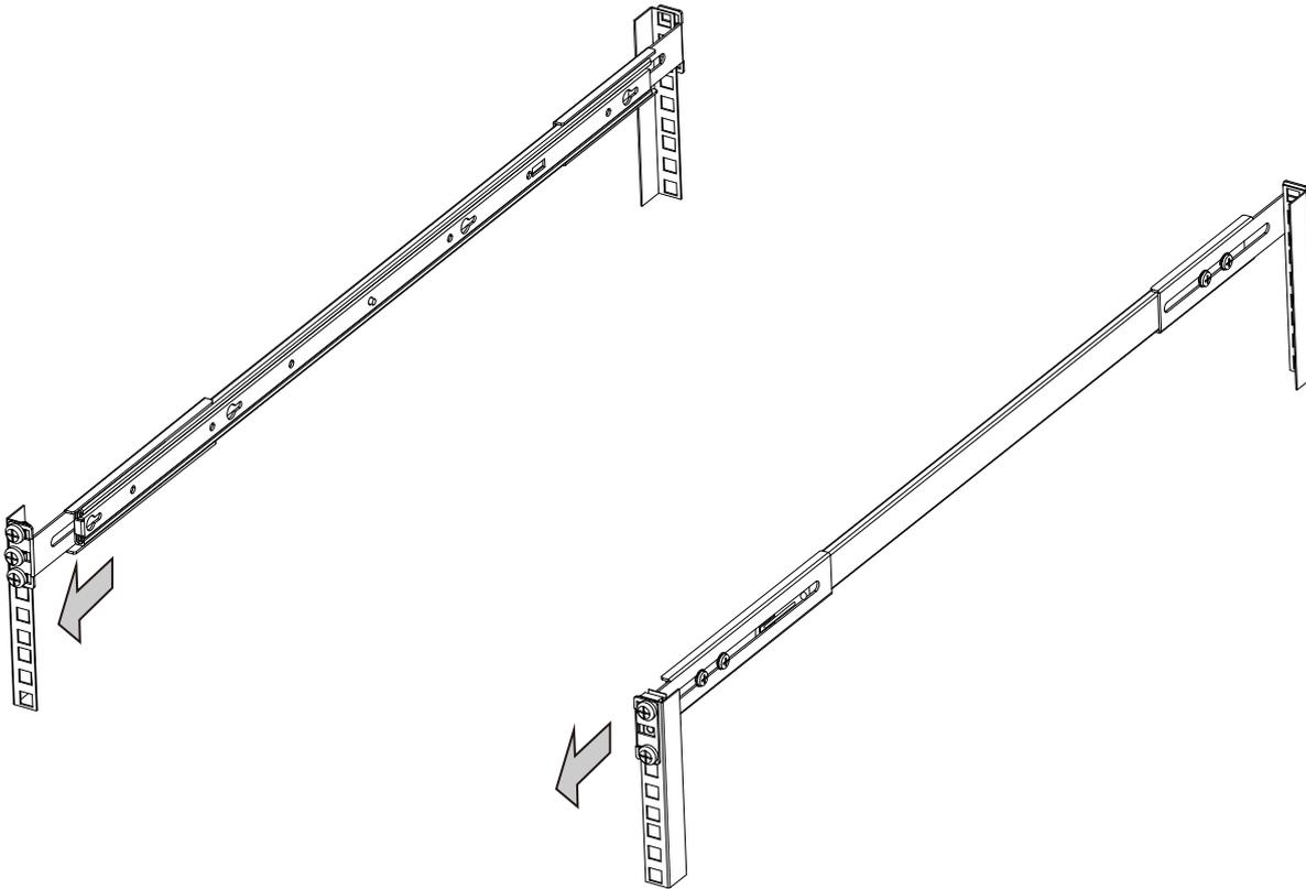
7. Hold the chassis using both hands on the sides of the chassis. Align the tips of inner rails on the chassis with the open portion of the slide rail assemblies. Push the system into the assemblies until the system stops.
