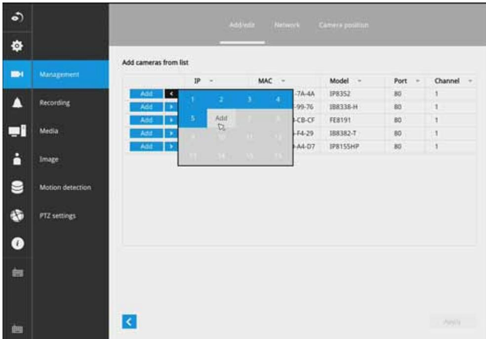
2. Click the **Add** button, the camera will be placed at an unoccupied position. You may also expand the menu on the side of the Add button to select a position number.
