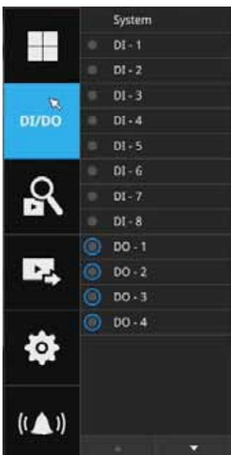
Click on the DI/DO button to display the full list of all DI and DO signals (whether they are connected or not) from all cameras in the configuration. If a digital input signal is triggered, e.g., the DI-4 on the left, its indicator will turn solid white.
