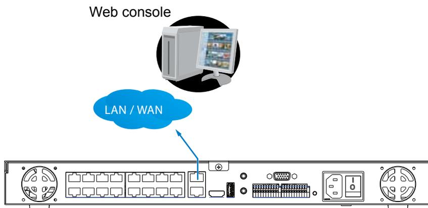
Note that when accessed over the network, the total streaming throughput is 96Mbps.
