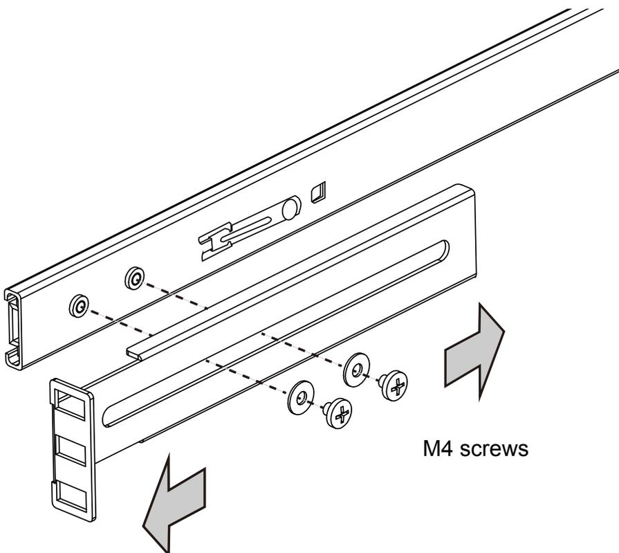
Adjust the length of rails to match the rack posts.
