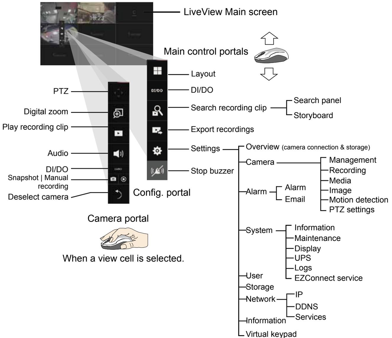
After you finish configuring using a Camera portal, click again on the camera view cell to reveal the main control portals.
