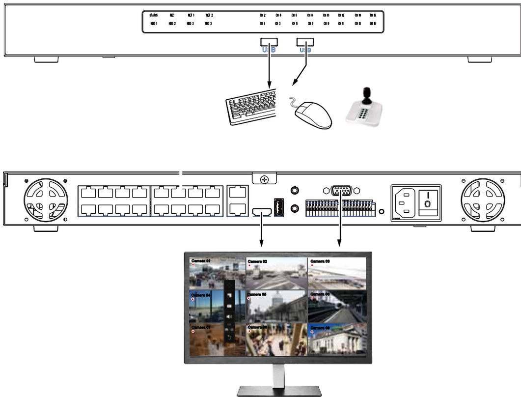
By default, a live view appears on an HDMI monitor. The interface architecture of the local console is illustrated as follows:
