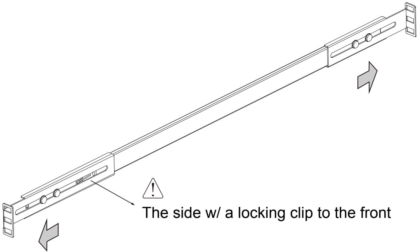
5. Secure the slide rails to rack posts using the #10 screws.
