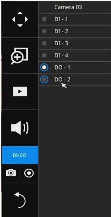
The DI/DO panel provides a glimpse of all DI and DO signal statuses from the connected cameras. You can manually trigger a digital output by clicking on its indicators.
