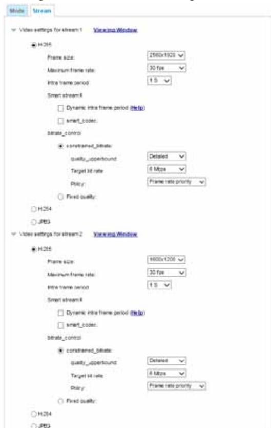
This Network Camera offers real-time H.265, H.264, and MJPEG compression standards (Triple Codec) for real-time viewing. If the **H.264** or **H.265** mode is selected, the video is streamed via the RTSP protocol. There are several parameters through which you can adjust the video performance:
