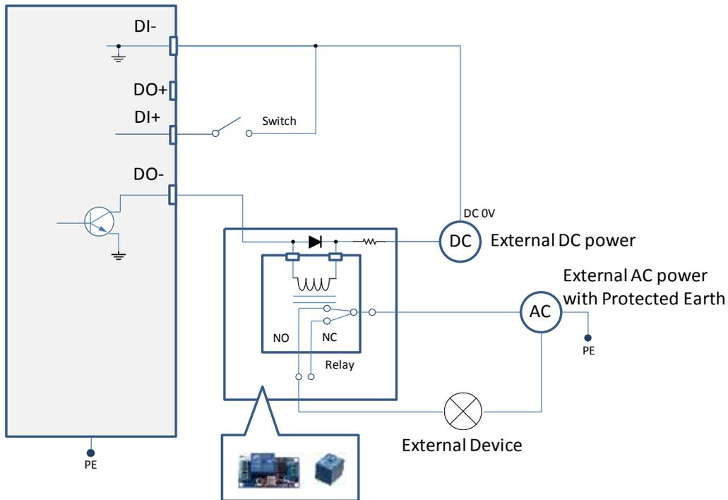
Dry contact and using camera's DO+ to supply a relay.
