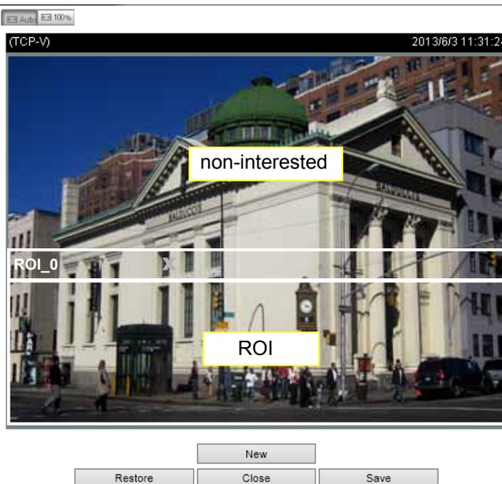
As the result, the lower screen is constantly displayed in high details, while the upper half is transmitted using a lower-quality format. Although the upper half is transmitted using a lower quality format, you still have an awareness of what is happening on the whole screen.
