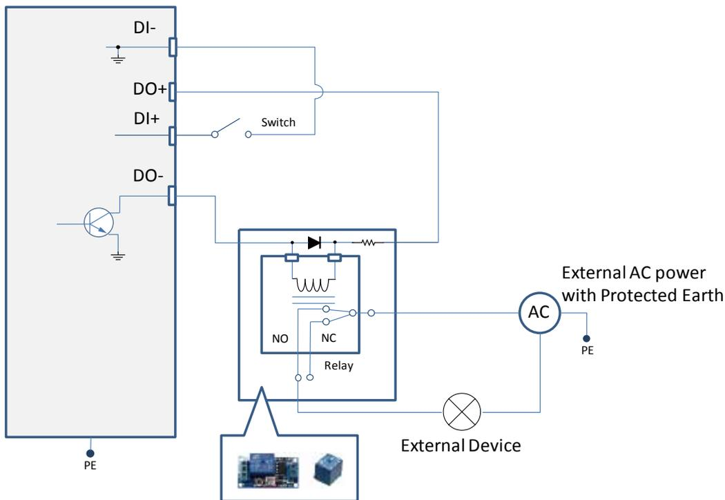
1. The DO+ pin provides 5V output voltage, and the max. load is 50mA.
