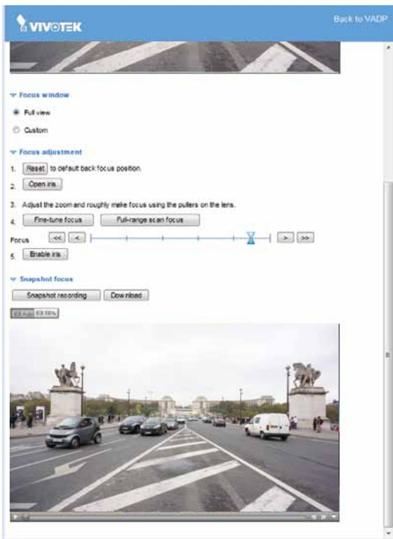
2. The recording takes place on Stream 1 with a focusing result calculated from the full of the current field of view.
