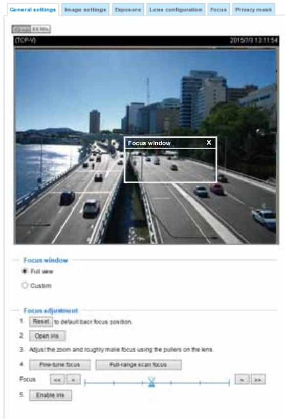
Below is the procedure to perform the automated Focus function:
