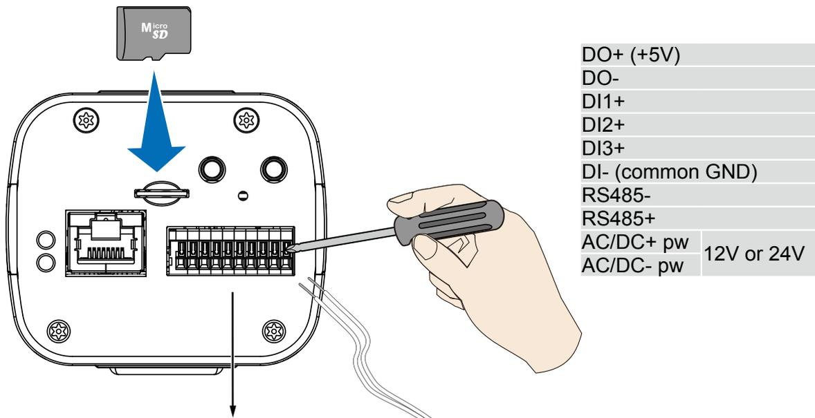
The DO pin can provide a 5V output, and the max. load is 50mA.
