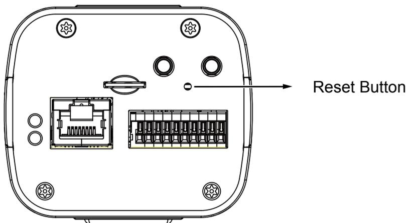
The reset button is used to reset the system or restore the factory default settings. Sometimes resetting the system can return the camera to normal operation. If the system problems remain after reset, restore the factory settings and install again.
