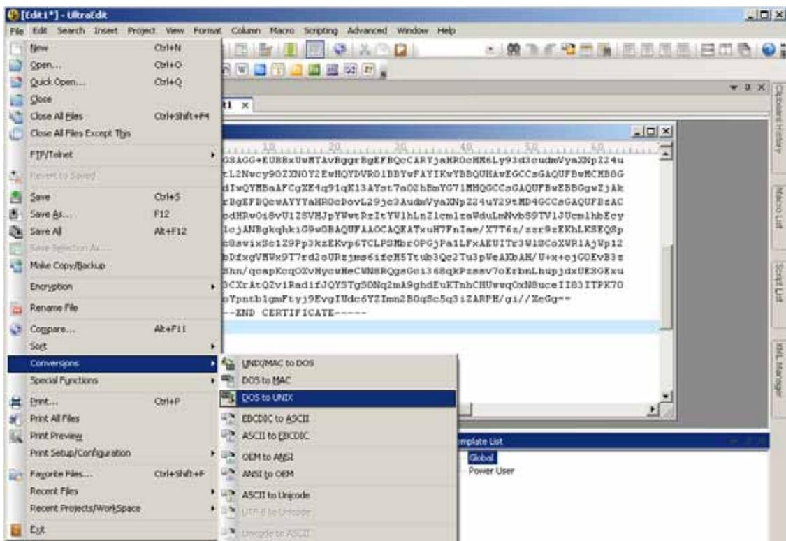
9. Save the edit using the “.crt” extension, using a file name like “CAcert.crt.”
