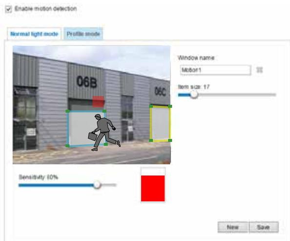
The Percentage Indicator will rise or fall depending on the variation between sequential images. When motions are detected by the Network Camera and are considered to exceed the preset threshold, the red bar rises. Meanwhile, the motion detection window will be outlined in red.
