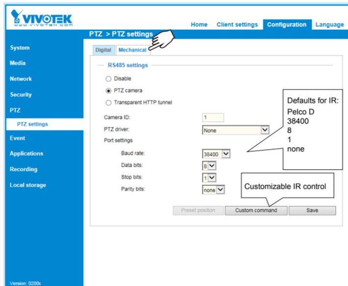
You can create custom buttons on a web console, such as IR brightness (Lux), threshold, dimming, etc.
