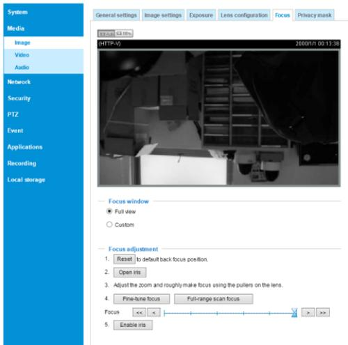
In the Configuration > Media > Image settings page, select an application scenario, LPC Highway, street, or parking lot mode. The related parameters, such as shutter time, will be automatically changed for the scenario.
