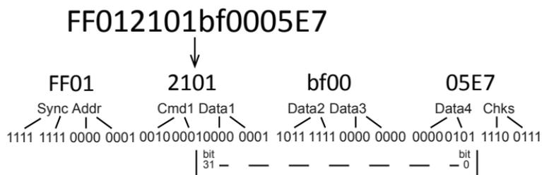
The format uses Hexadecimal 0-9, A-F. Each 8-bit byte contains two 4-bit hexadecimal characters. Two hexadecimal characters contained in each 8-bit field of message.
