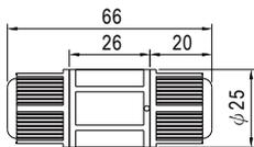
CJ04-1 suitable for 14AWG~16AWG
