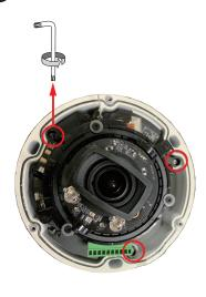
Use 2 seal rings when installing the conduit.
