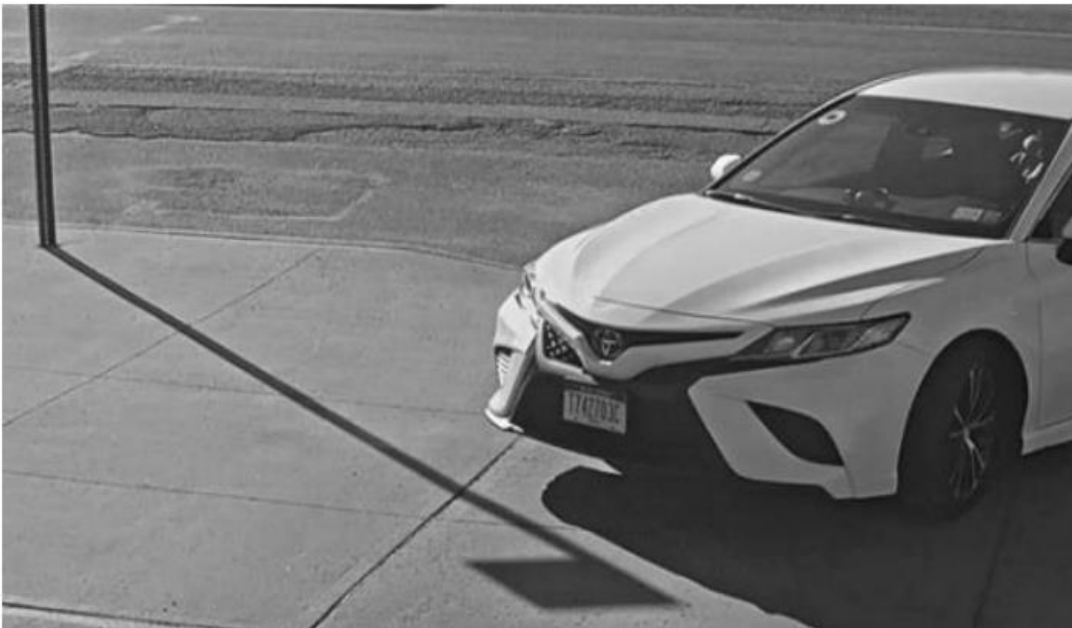
INCORRECT: Access control, horizontal angle too acute
