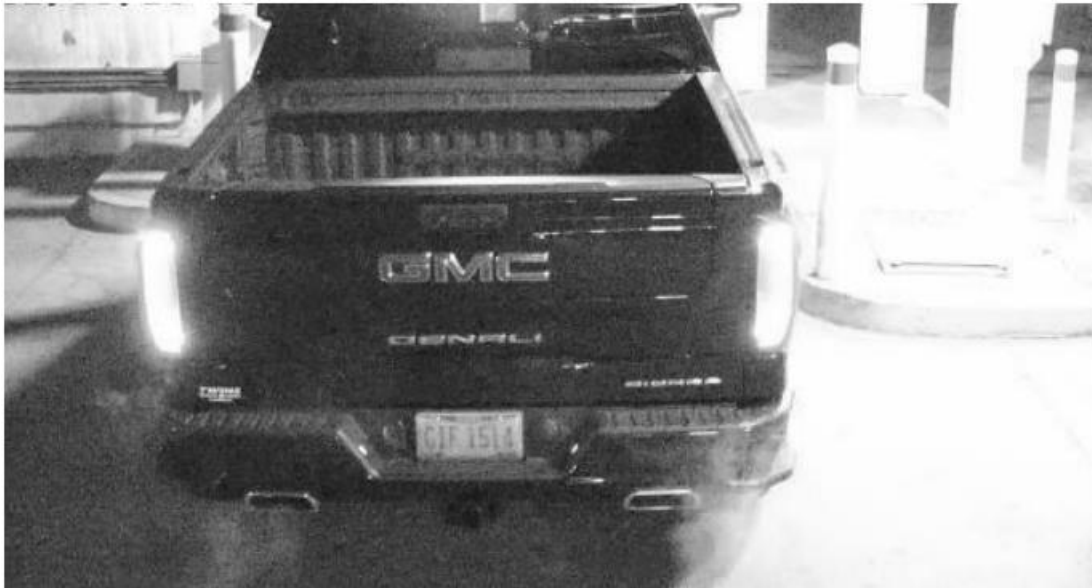
INCORRECT: Access control, good camera position, bad quality images
