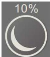
Turn LED on when ambient light is under 10 % and turn off when the ambient light is above 20 %.
