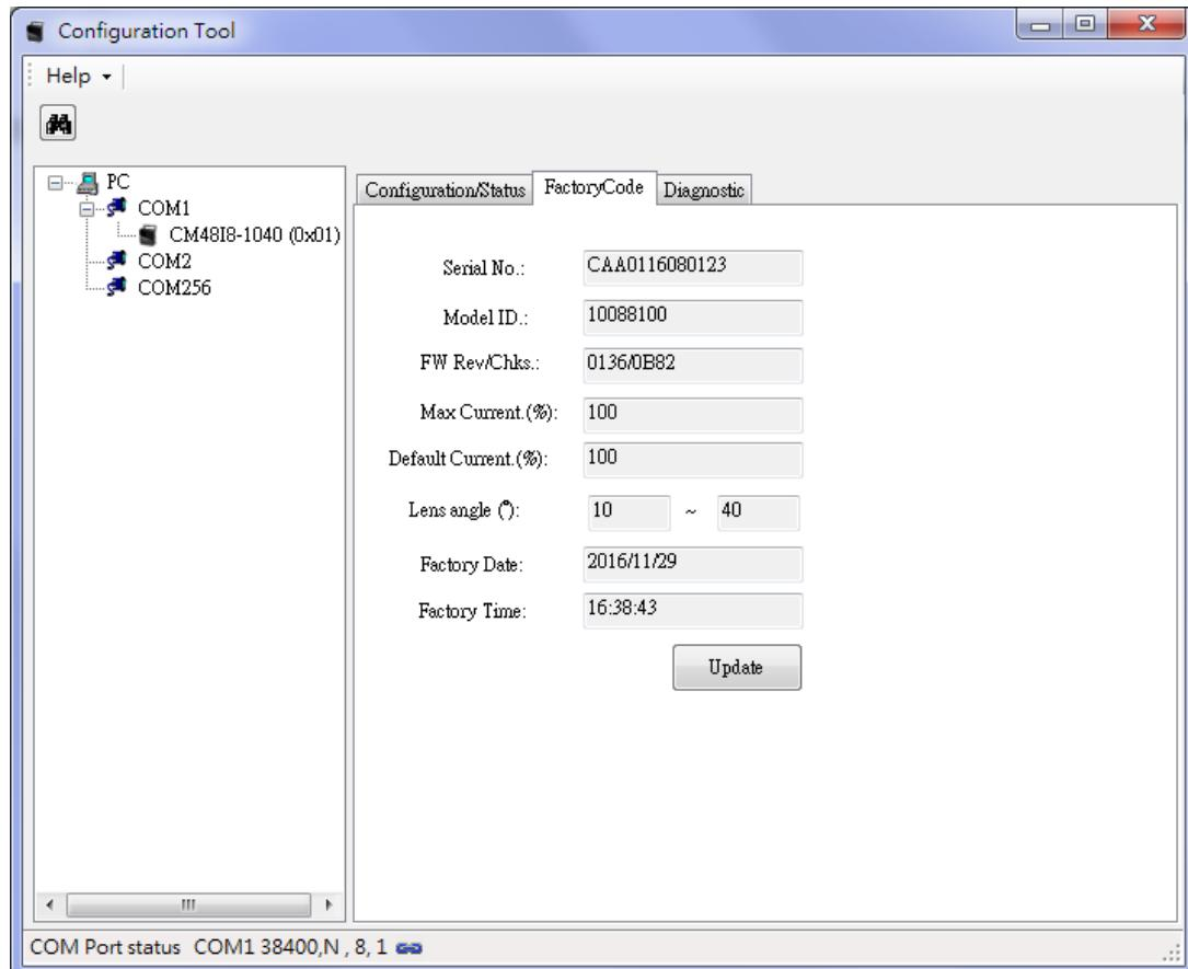
The FactoryCode page records manufacturing information of the device. Generally, the code is used for manufacturing.
