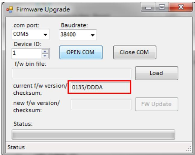
If the software cannot connect to a CaMate, a timeout warning displays. Please check if the COM port and/or baudrate settings are correct, or the wire connection is correctly made.
