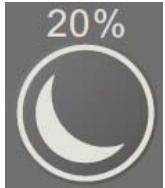
Turn LED on when ambient light is under 20 % and turn off when the ambient light is above 30 %.
