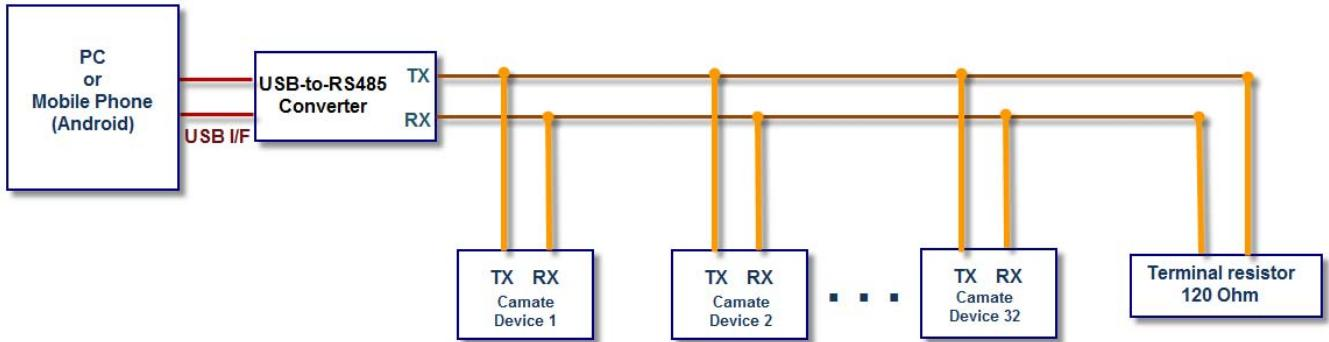
NOTES: If termination is required, a resistor value of  $120\Omega$  or greater should be used, and no more than 2 termination resistors should be used, one at each end of the RS485 transmission line.
