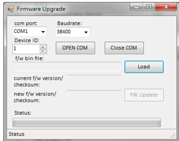
1. Select the correct COM port, Baudrate, and Device ID, then click the OPEN COM button. When a CaMate is connected, current firmware version and checksum will be read and shown.
