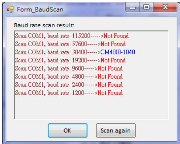
2. Then, configure the correct baudrate and click the Find icon. A search device window will prompt to ask for a start Device ID number. Default is 1. Unless a change to the device ID of your CaMate was made, otherwise, press OK to start finding from device ID 1. You can press the Stop scan button any time once your CaMate is found.
