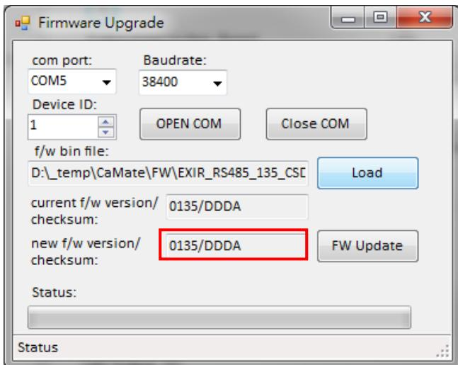
3. Click FW Update and confirm the upload, firmware upgrade will then start. Please do not turn off the power to CaMate until the upgrade is completed.
