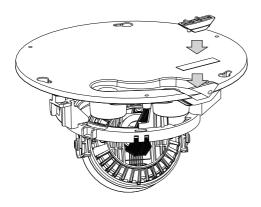
3-2-2. Install the camera to the mounting cap by turning it counter-clockwise so that the screw heads fit in the keyhole slots. Fasten the screws, and then connect the cables.
