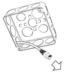
2. Install the mount cap to the junction box. Use screw holes specified on page 3 depending on the type of junction box.
