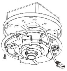
3-1-2. Connect the cables and install the top cover.
