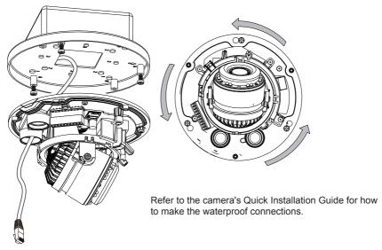
3-2-3. Install the dome cover. Tune the focus, and refer to the documentation that came with your cameras for the rest of configuration details.
