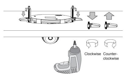
10. Adjust the shooting angle and check for a satisfactory image over a web session. When you have a satisifactory live view, tighten the tilt screw, and secure the dome cover from below the ceiling using the T10 stardriver.
