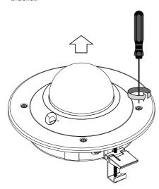
5. Remove the breakaway tab from the bottom of the camera so that you can route cables through the opening.
