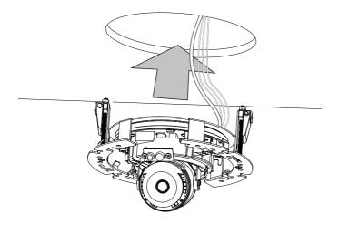
9. Use a #2 Phillips screwdriver to move the clamping plates down so that the ceiling/board is caught between the clamps and the flange on the other side of the ceiling.
