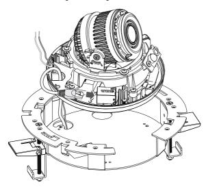
8. Use a #2 Phillips screwdriver to loosen the clamping plates (see drawing below) and insert the recessed-mount bracket through the hole in the ceiling.
