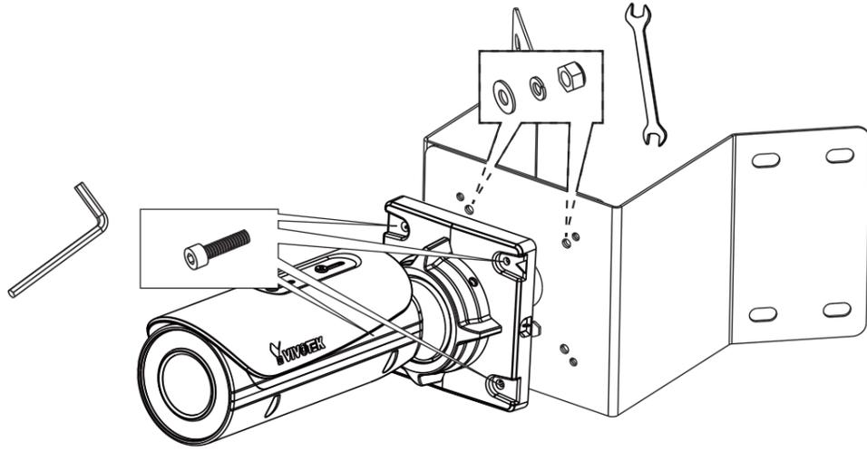
The installation of IB8367A, IB8369A, IB8377, IB8379, and IB9389 is similar to the above, except using different mounting holes and screws.
