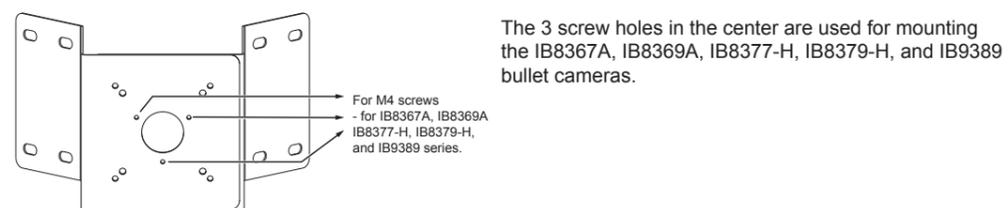
The 3 screw holes in the center are used for mounting the IB8367A, IB8369A, IB8377-H, IB8379-H, and IB9389 bullet cameras.
