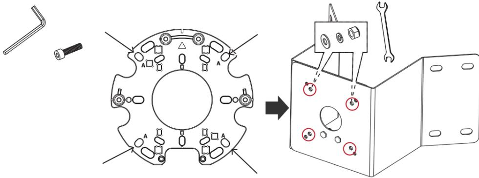
Below are the corresponding mount holes for the MS9390-HV.
