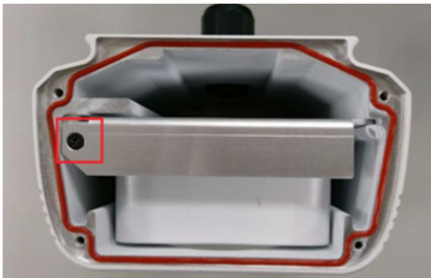
19. Tighten up the cable gland, adjust the cable length, and install the side cover.
