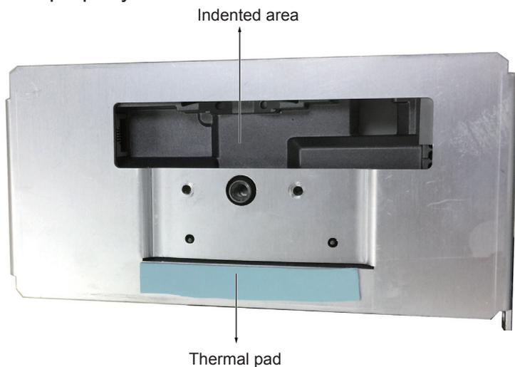
14. Secure the slide bracket to camera using 2 M3 screws.
