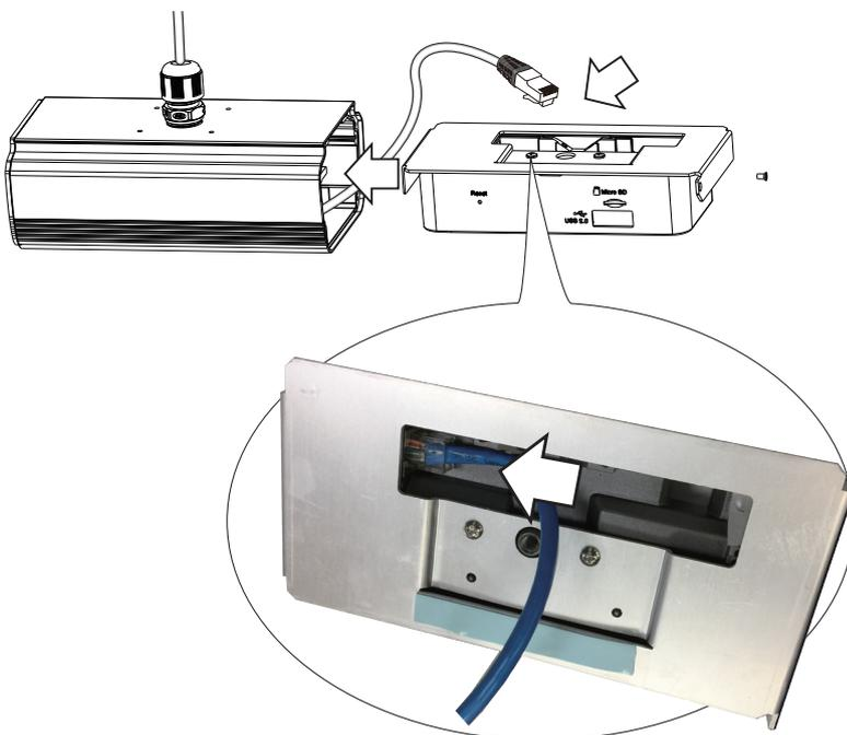
18. Secure the slide bracket by driving an M3 screw.
