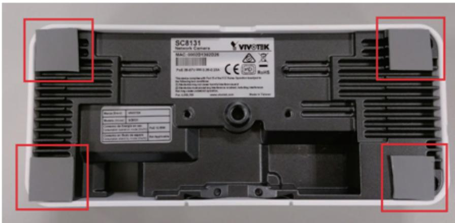
13. Place the slide bracket on top of the camera. The opening should provide access to the indented area on the back of the camera. Make sure another long piece of thermal pad is properly installed on the slide bracket.
