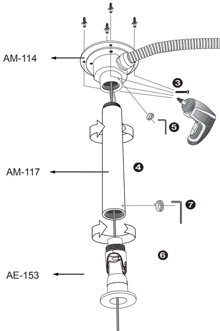
8. Prepare the AE-153 bracket components. The components are shown below:
