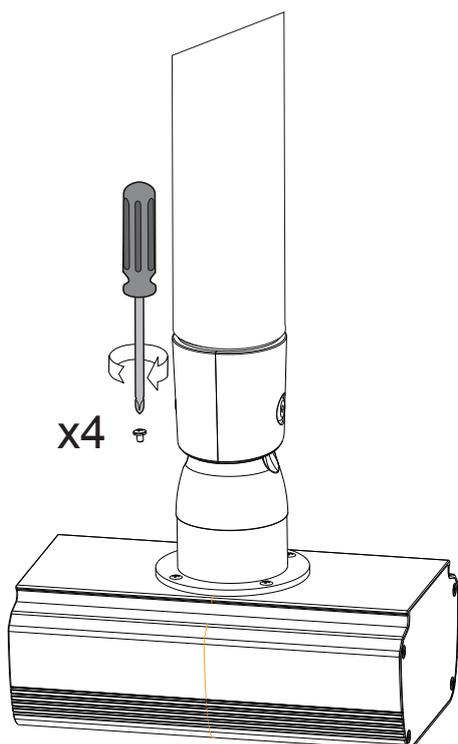
21. Loosen the hex socket crew and adjust the orientation, the shooting angle, or the tilt angle if necessary.
