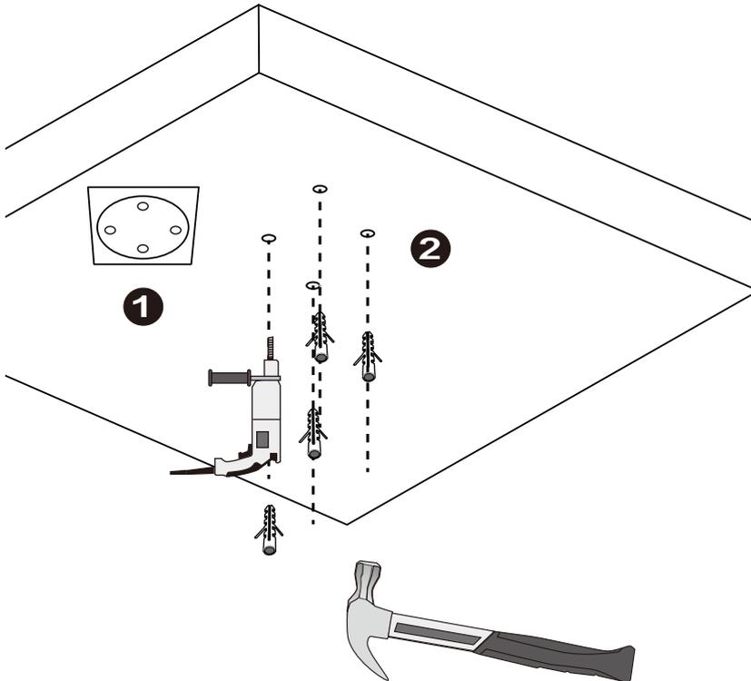
3. Secure the pendant head using the included screws.
