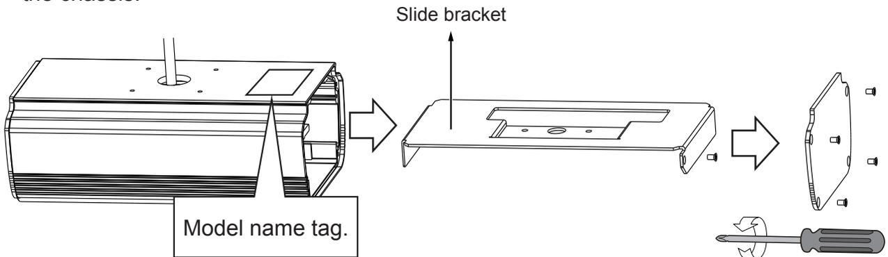
11. Remove two retention screws from the back of camera.
