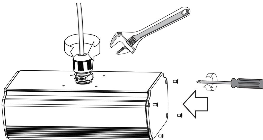
20. Secure the chassis to bracket by driving 4 M3 screws.
