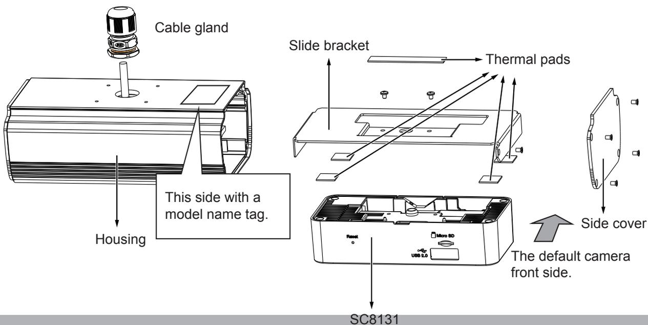
9. Route a CAT5e Ethernet cable through the pendant pipe, and install the cable gland components to the Ethernet cable.
